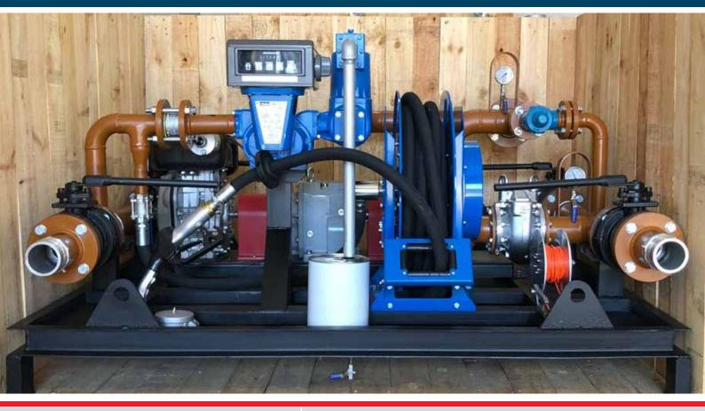
Capable of down-loading, uploading and circulating Diesel fuel at 500 l/min without the need of disconnection or reconnection of site hoses.
